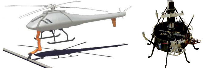
Fig. 2. Examples of UAVs endowed with a manipulator: on the left the ARCAS-project concept; on the right the AIRobots-project prototype.
