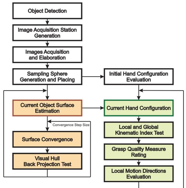
Fig. 1. Block diagram of the visual grasp algorithm.
