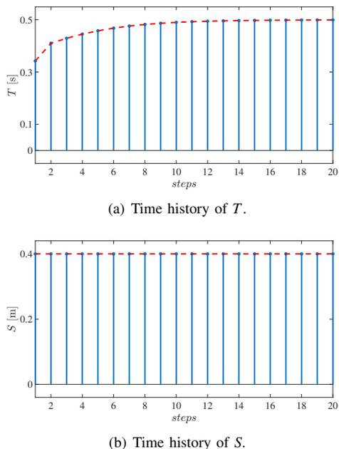
Fig. 3. Case Study I, step period  $T$  and step length  $S$ . Blue bars: the step-by-step evolution of (a)  $T$  and (b)  $S$ . The red lines show that  $T$  and  $S$  converge to their target values 0.5 s and 0.4 m, respectively.
