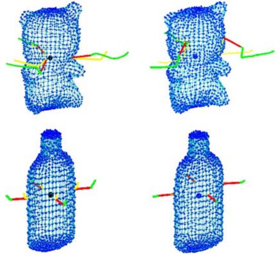
Fig. 11. Trajectories of the fingers (green: approach with safety distance  $\delta_f$ , red: grasp) and corresponding sequence of points computed by the grasp planner (yellow) for the two objects, evaluated with  $k_{c_m} = 1$  (left) and  $k_{c_m} = 0$  (right).
