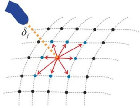
Fig. 7. Possible displacements from the current grasp point.
