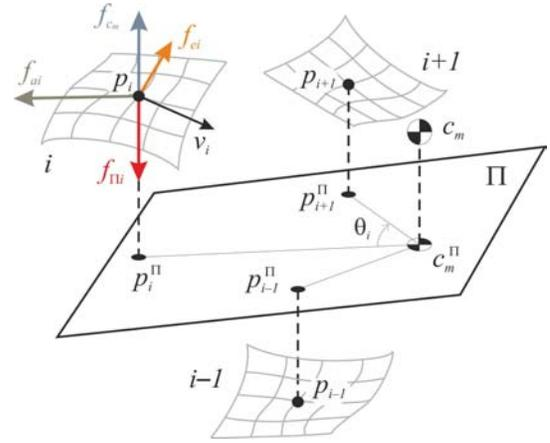
Fig. 8. Forces at contact point  $\mathbf{p}_i$ .
