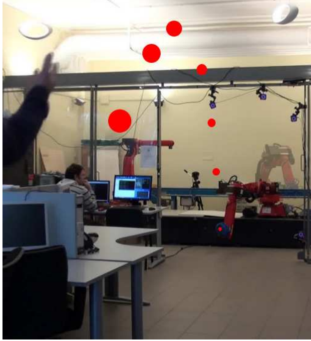
Figure 5: Overlay of the ball trajectory and robot motion.
